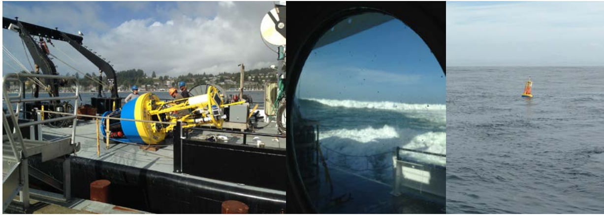
Figure 2: The NewH10 MAPCO2 mooring, developed and built at OSU-CEOAS. Left, populated mooring ready for deployment on deck of OSU's RV Oceanus ; middle, crossing the bar in 20' seastates; right, deployed mooring at NH10.
