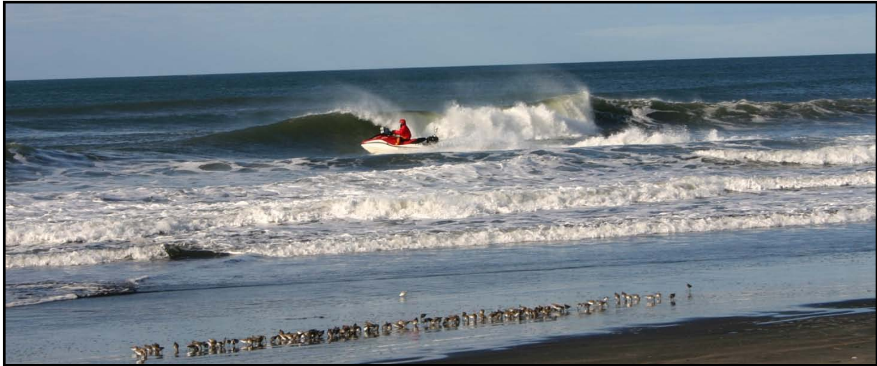
Figure 17. 4 th generation Coastal Profiling System collecting nearshore bathymetric data.
