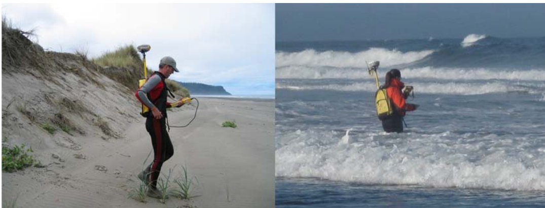
Figure 14: Beach profile surveys being undertaken using a Trimble R8 GPS rover mounted on a backpack.
