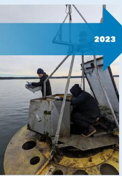
An ORCA buoy in 2023 with 15 years of grime, corrosion, and bird poop
