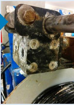
Vital buoy winch parts wear out from being in a seawater environment 24 x 7 x 365
