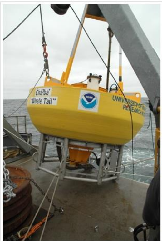
IOOS partners in the Northwest Association of Networked Ocean Observing Systems (NANOOS) deployed this buoy in 2010 as part of a three-piece observing array to assess issues in the Northwest, including ocean acidification, hypoxia and harmful algal blooms , and climate change . The coastal buoy will aid computer models that predict ocean and atmospheric conditions. Known as "Chá bã," the buoy is named for the Native American word (pronounced "chay buh") for "whale tail."
