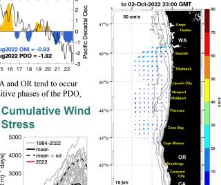
127°W 126°W 125°W 124°W 123°W Primary currents flow north and south in winter and summer, respectively, except within ~10 km of shore, where fluctuations follow changes in wind direction.
